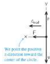
(b) Free-body diagram for pendulum bob
